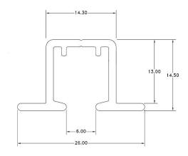
The Martec "High Line" (Recessed Track) is designed to fit into a cut-out in the ceiling GIB so that it sits flush with the ceiling.
